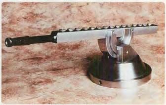
With its casing removed, the single-barreled prototype's 15 external priming ports, in which ball powder is loaded, are visible along the top of the barrel. Note the difference in effective barrel length between the first and last rounds of the payload; this can affect a projectile's ballistic performance.
